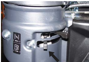
Gasoline Shut Off Valve (Shown in off position)
